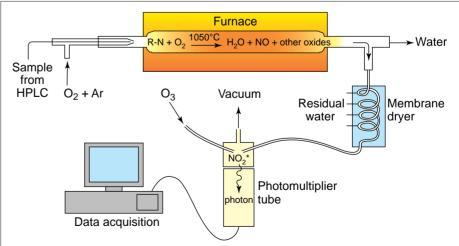
**Figure 1.** Working principles of Antek Model 8060 – a chemiluminescence nitrogen detector. NO<sub>2</sub>\* indicates NO<sub>2</sub> in its excited state.
